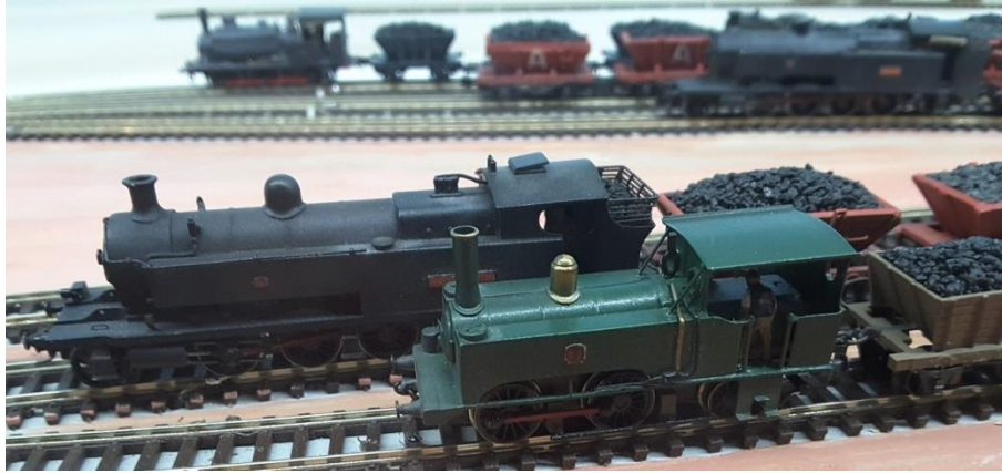
J&A Brown loco #1, 1856 Hawthorn built 0-4-2; and J&A Brown loco #10 "Richmond Main", 1911 Kitson built 2-8-2; both DCC scratch built by Stephen CURRY
