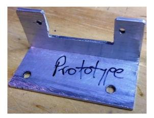
Along a strip of 20mm aluminium angle, a series of brackets were scribed, and centre punched ready for drilling and cutting.
