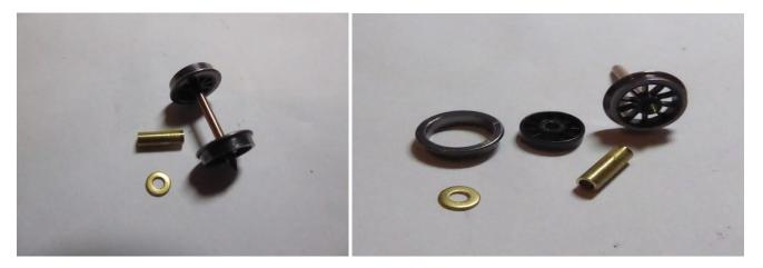
The brass tube is the pickup; it should spin freely on the axle. The washer protects the wire from the end of the tube. All that remains is to route the wires from the power supply to the brass sleeves.
