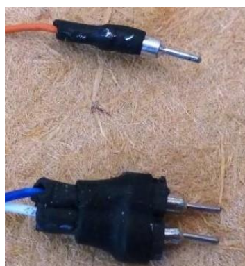
Wiring to small IC pin/socket connectors, ideal for steam loco to tender connections
