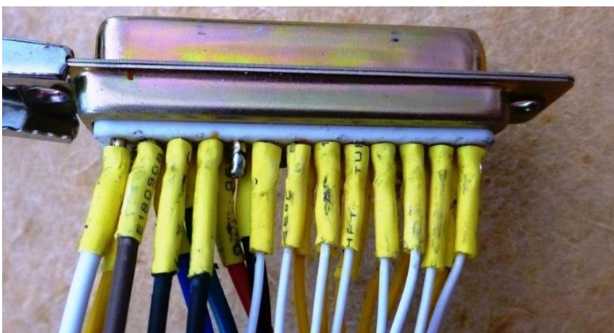
Wiring to small IC pin/socket connectors, ideal for steam loco to tender connections
