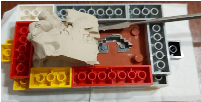
1 st pour of the BARNES RTV allow 24 hours to set
