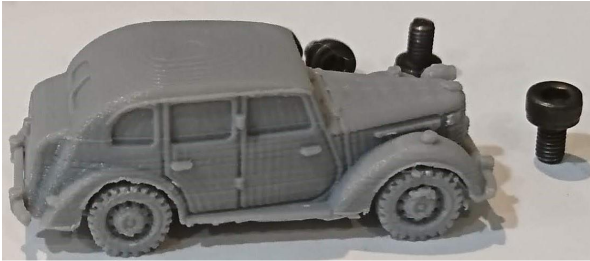
Austin 10 fresh off the printer before flash removal & painting.
