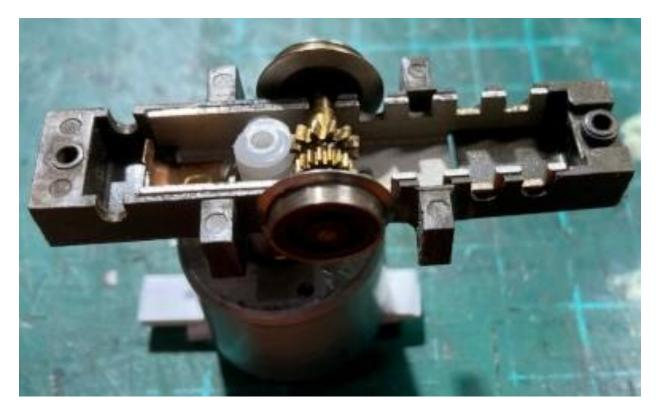
The motor sits on the truck and just clears the chassis. The decoder and required keep-alive fit nicely in the middle of the body (there are only 5 live wheels in total, 2+3.)
