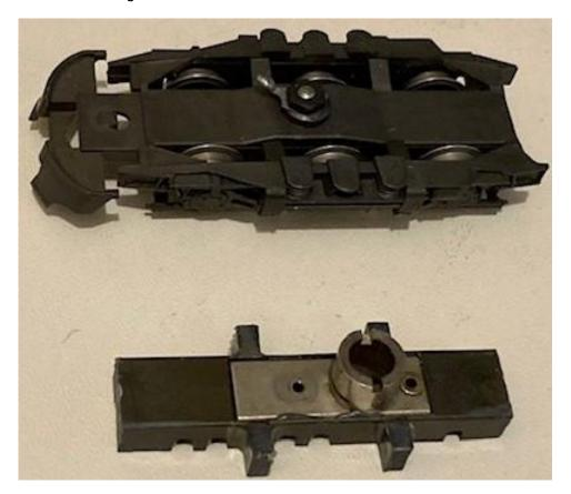
A round brass shim provides a snug fit for the motor, which cannot be attached to the truck until the truck is attached to the chassis & of course the side frames had to be replaced with the 47 class provided with the kit.
