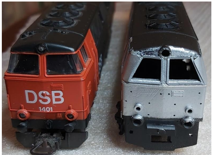
Lower right: MZ modified windscreen and deflectors
