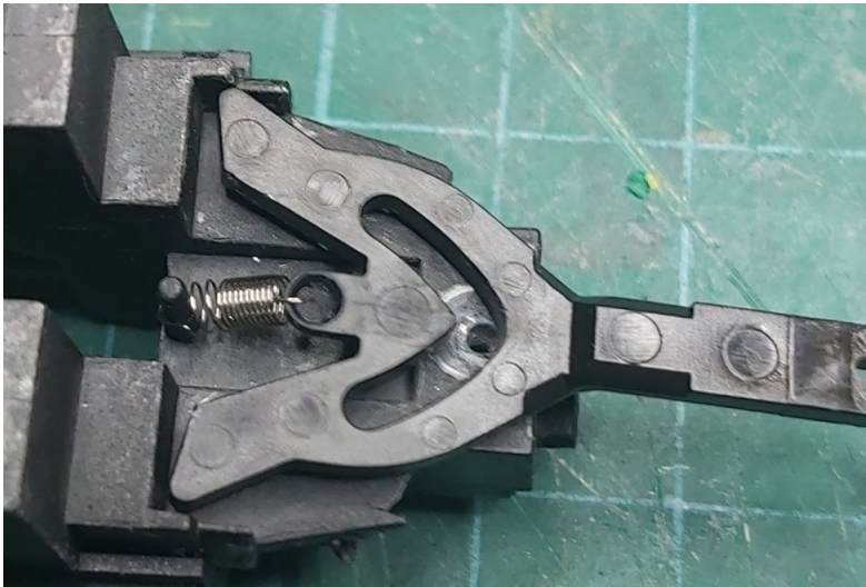
Application of graphite & securing with a 2-56 screw and fibre washer.
