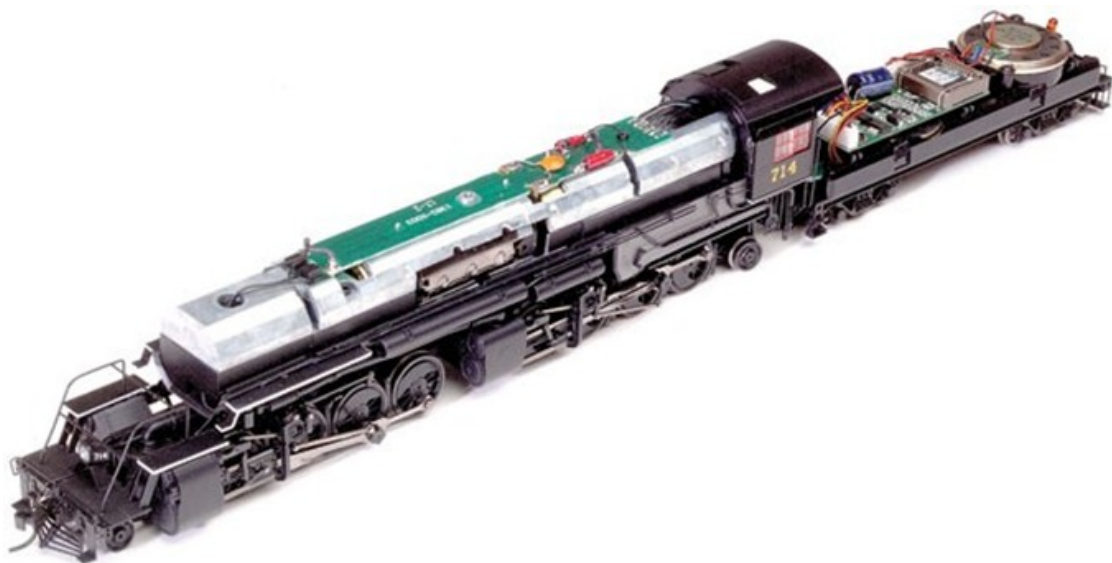
Web picture of the boiler top removed showing a DCC board.
