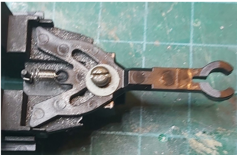
Application of graphite & securing with a 2-56 screw and fibre washer.
