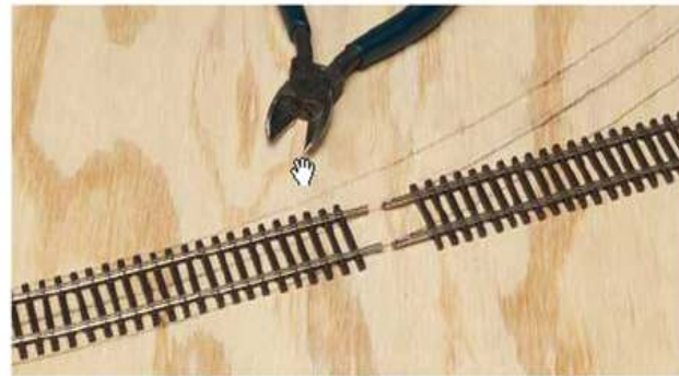
The Atlas code 83 H0 flextrack at left is laid on a 26" radius, except for the last three inches. After trimming the rails on that section for a square joint, Andy Sperandio is ready to add a new section that's still straight. Bill Zuback photos
