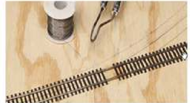
Andy has joined the two sections with rail joiners, and soldered the joiners with the rails still straight through the joint. Small-diameter resin-core solder makes it easier to make a neat, strong joint without building up excess solder.
