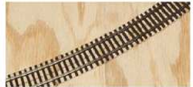
Now the joined sections are bent to the 26" radius with a smooth curve through the joint. Andy saves extra ties to fill gaps in the tie strip, and always cleans the joints with denatured alcohol to keep excess flux off wheels and railheads.
